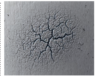
Only high power transient loading damaged the tungsten surface (3 x 3 mm).
