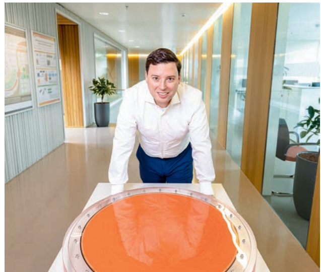
Matthijs van Berkel with a rheoscopic disc, build to visualize turbulence.
