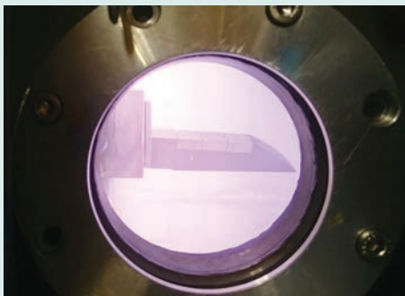
Exposing a misaligned tungsten block to the plasma in Pilot-PSI (left) reveals an increased heat load on exposed leading edges (IR-view, right)
