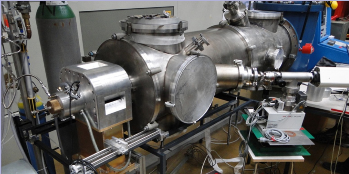
Above: Solar Fuels test facility with microwave-plasma reactor and diagnostics.
