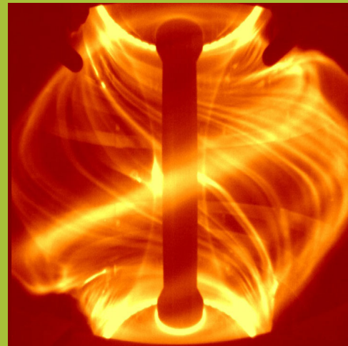
Edge Localised Modes in the MAST tokamak produce high transient heat loads on plasma facing materials
