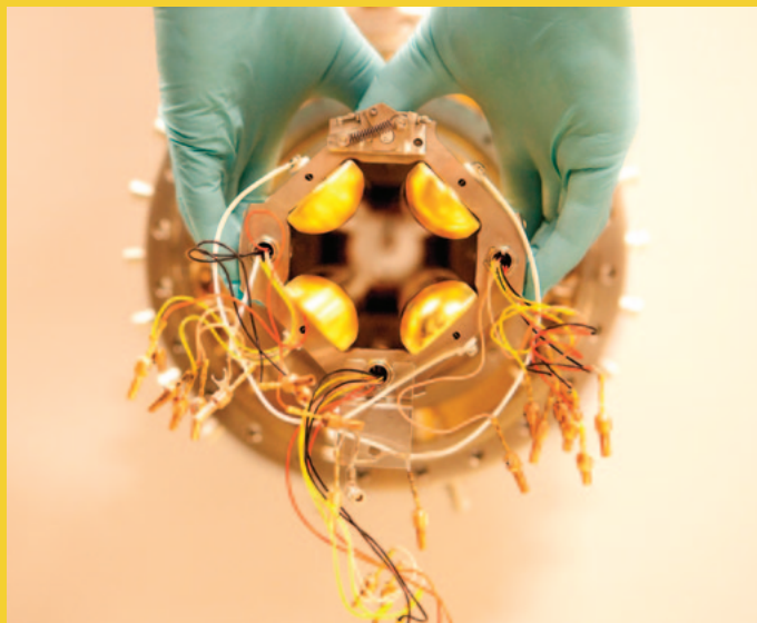
Figure 2.24 Close-up of the quadrupole ion guide that transfers the ions into the ICR cells of the second FELICE experiment, the FTICR mass spectrometer.
